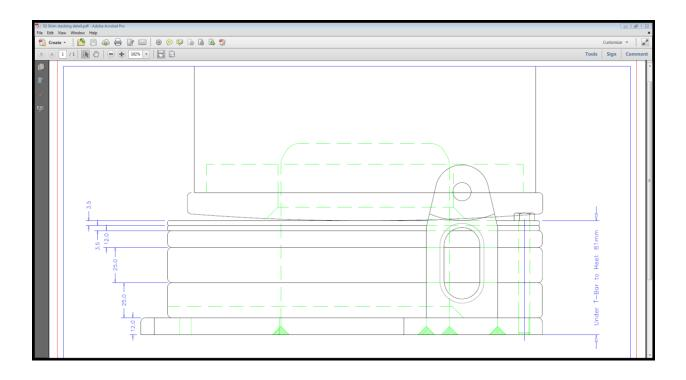
19.13 TOP OF POLE TRACK – The top of the spinnaker pole track shall be not less than 2630 mm or more than 2638 from the top of the lower band.
